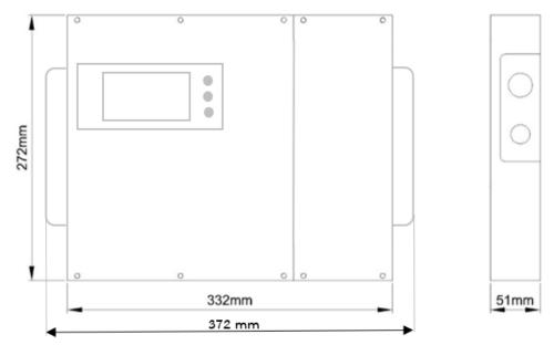
We are recommend fixing to height ranging between 1.50m and 1.8 m to allow a comfortable height to see the display.
